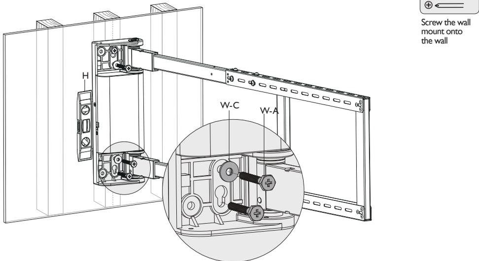
Screw the wall mount onto the wall
