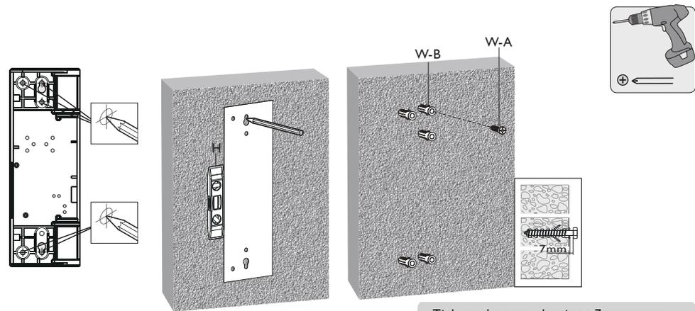
Tighten the screw leaving a 7mm space from the wall.
