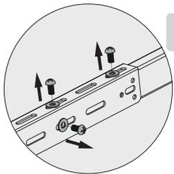
Remove the screws and washers using the proper phillips screwdriver.
