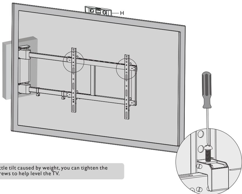
To avoid the little tilt caused by weight, you can tighten the adjustment screws to help level the TV.
