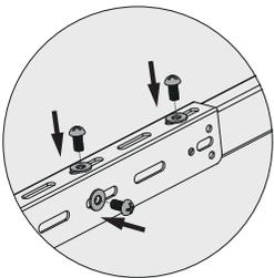
Reinstalling the screws and washers to secure the swing arm after finishing the adjustment.
