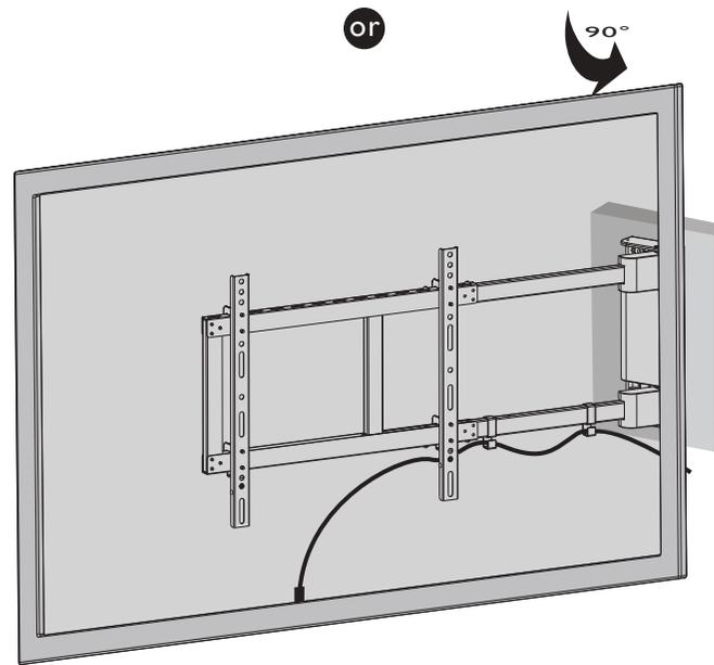
Connect the cables to your TV and route through the cable clips.
