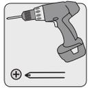
Tighten the screw leaving a 7mm space from the wall.
